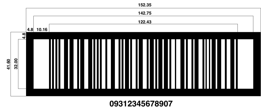
Nominal (100%) Magnification ITF-14 Barcode (not to scale)
